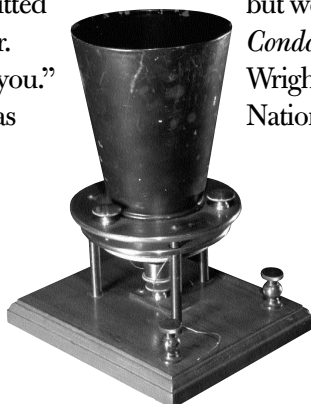
Bell’s liquid (variable-resistance) telephone transmitter
